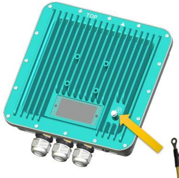
Connect one of a grounding cable to the grounding screw and firmly tighten the grounding screw. Connect the opposite end of the grounding cable to a good ground(earth) connection.
